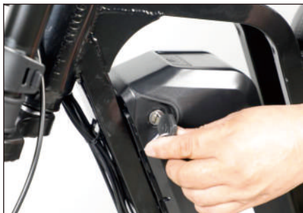
❶ Battery Keyhole (Insert the Key)
