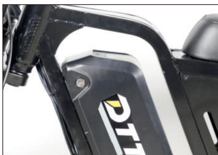
❻ When charging is complete, place the Battery properly, insert the key, and rotate it clockwise to secure the Battery.
